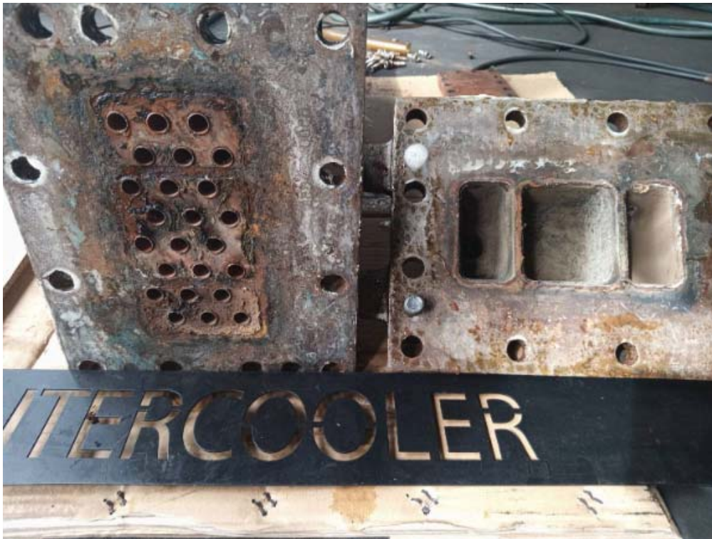
INTERCOOLER BEFORE CLEANING
