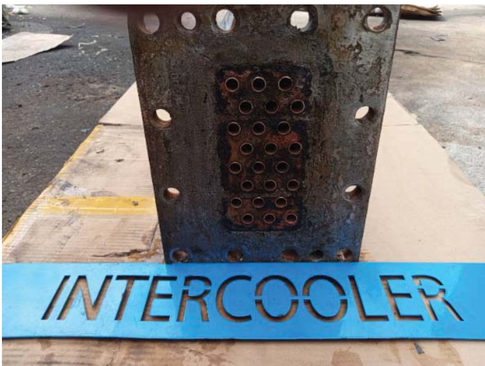
INTERCOOLER AFTER CLEANING
