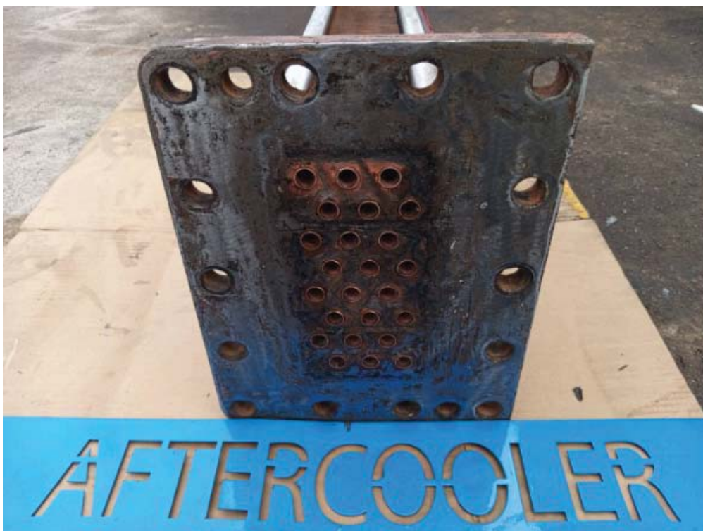
AFTERCOOLER AFTER CLEANING
