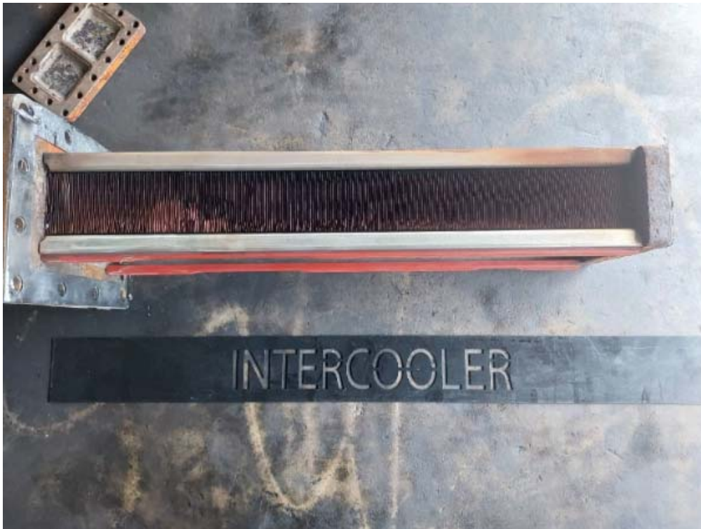
INTERCOOLER BEFORE CLEANING
