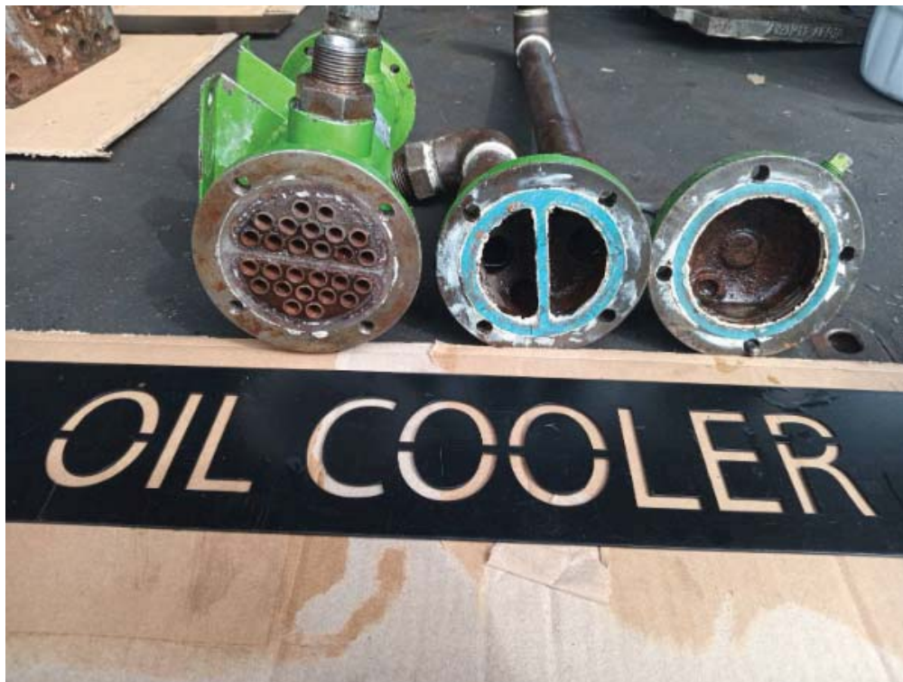
OIL COOLER BEFORE CLEANING
