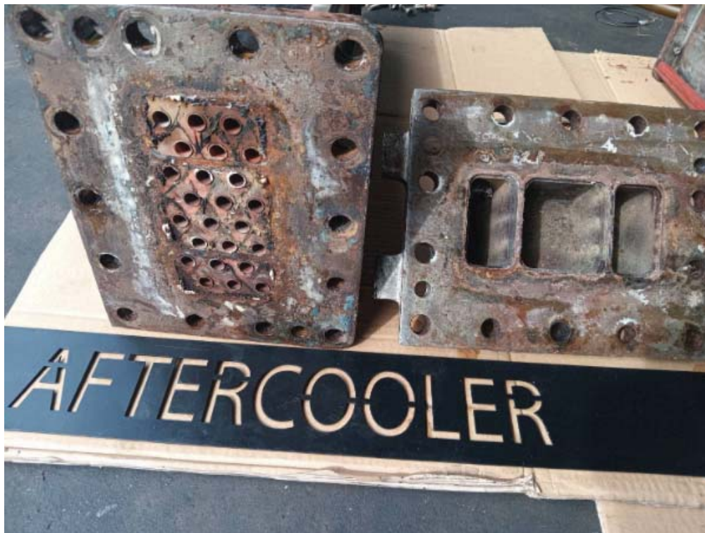
AFTERCOOLER BEFORE CLEANING
