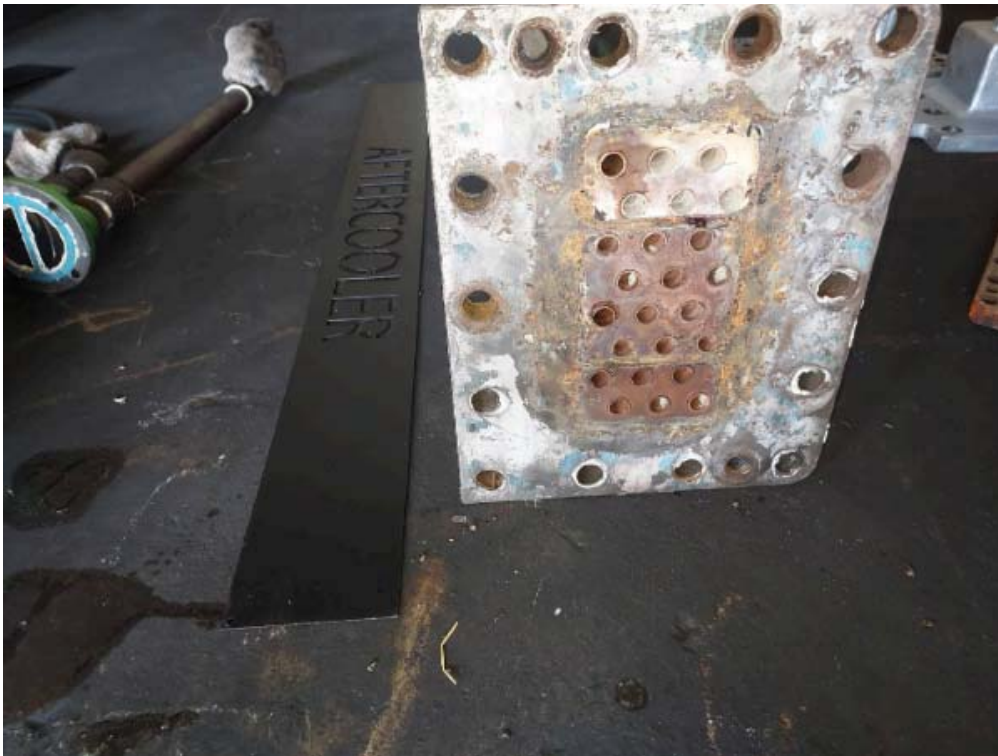
AFTERCOOLER BEFORE CLEANING
