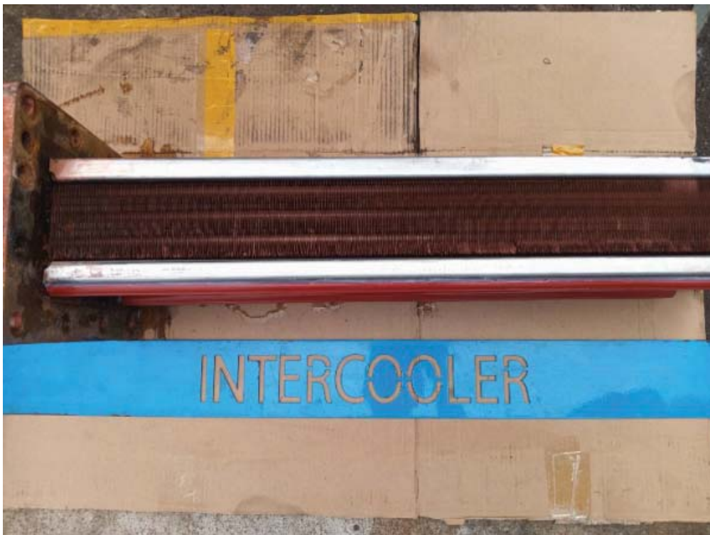
INTERCOOLER AFTER CLEANING
