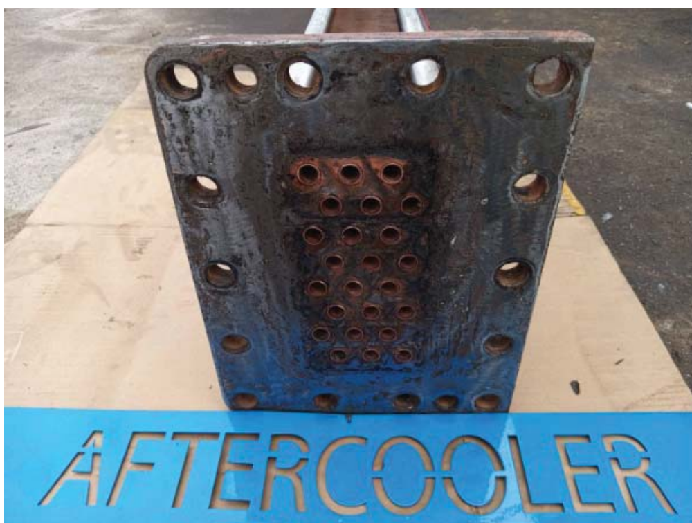
AFTERCOOLER AFTER CLEANING
