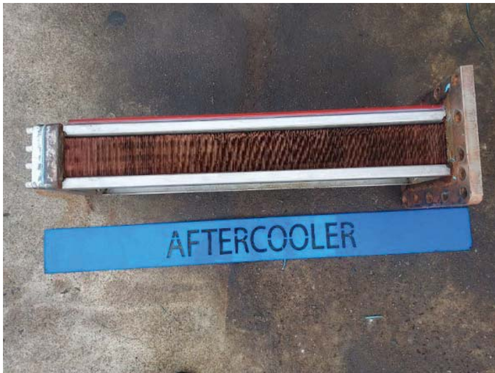
AFTERCOOLER AFTER CLEANING
