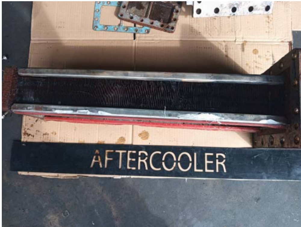
AFTERCOOLER BEFORE CLEANING
